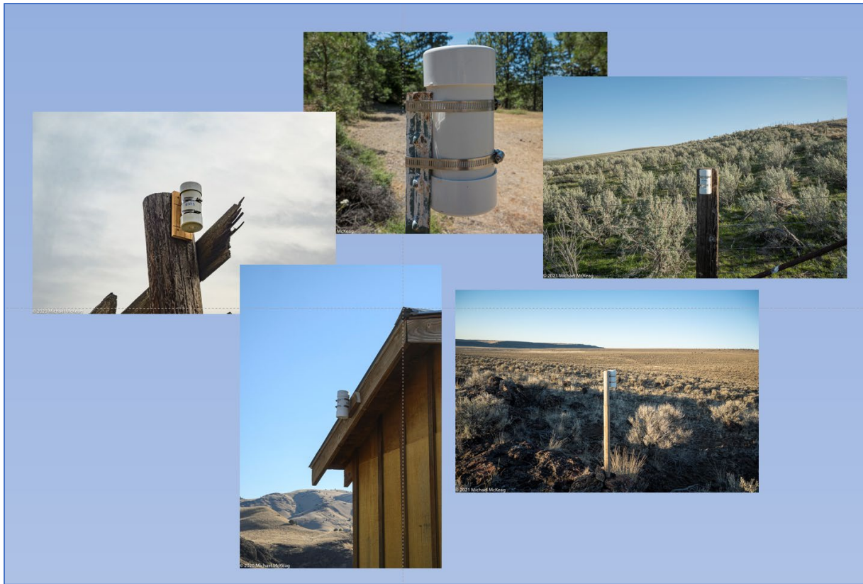
Figure 2. Examples of SQMs installed at sites in Oregon. The meter resides inside a weatherproof case and point vertically toward the sky.
